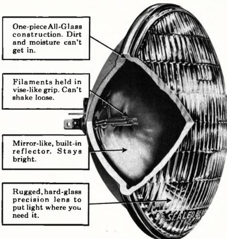
**WHEN YOU BLOW ON YOUR GLASSES**, moisture condenses on the lens. When moist air gets inside some types of sealed-beam headlamps, the same thing happens. It condenses on lens and reflector. And as the water deteriorates the reflector, the lamp grows dimmer.
