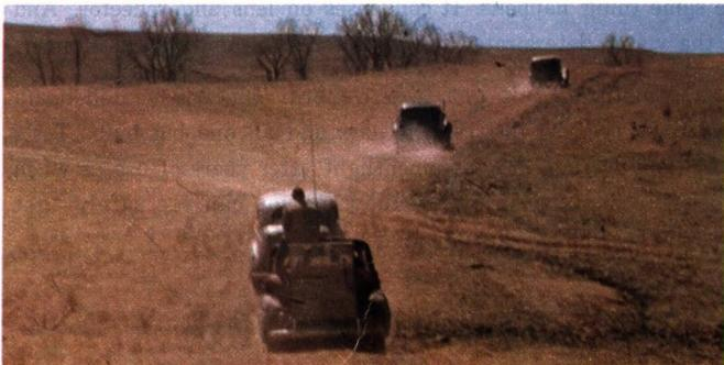
Jalopies roar over plains toward hunting area. Most have reinforced springs and doors welded shut to help them withstand terrific pounding of the chase
